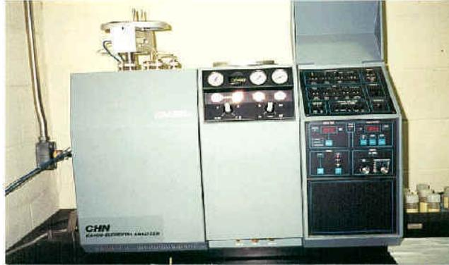
Fig. 5. C, H, and N analysis using the Elemental Analyzer E. A. 1108. The principle of analysis is the oxidation of the sample by "flash combustion".
