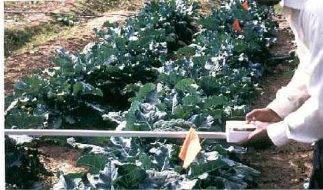
Fig. 2. Leaf Area Index (LAI) and percent canopy cover are measured with the AccuPAR. Here, photosynthetically Active Radiation (PAR) is measured above the canopy.
