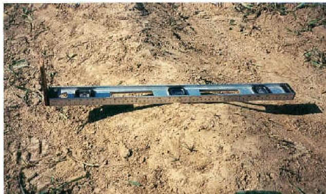
Fig. 1. Zenith angle is determined with the board/scale zenith angle device.
